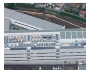
Photovoltaic power generation facilities on the rooftop of the new research building
